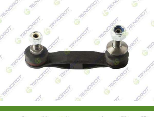
B-907 Suspension Stabilizer Bar Link Z-Rot Rear Arka 33556777635 coupling rod B=M10 x 1,5 H=M12 x 1,5 W=0,198
